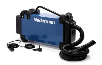
The Fume Eliminator is designed to be carried to the working area. Connected to a welding torch or to an extraction nozzle, the FE unit extracts the fume directly at source. FE 840 has a manual start/stop function while the FE 841 has an automatic start/stop function, which starts the unit as soon as the welding begins. Suitable for extraction of fume from maintenance welding applications.
