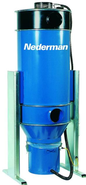
Dust collector with 2-stage filtration. Central inlet with velocity reducer. Fully automatic filter cleaning. Can easily be equipped with a great variety of filter materials, bins, emptying systems, etc. Standard equipped with circular bags of polypropylene. PTFE or antistatic filters on request.
