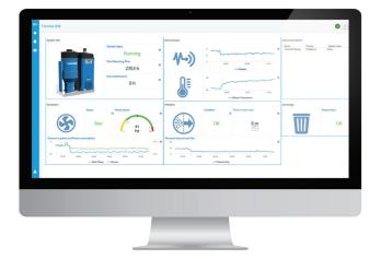
We have developed a cloud based IIoT\* platform designed specifically for filtration systems. It provides real time visualization and monitoring of system performance including customized dashboards and alarms.
