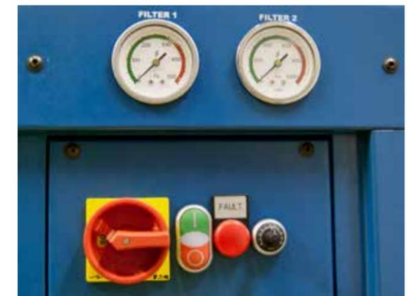
The FilterBench is equipped with pressure gauges clearly indicating when it is time to replace the filters.
